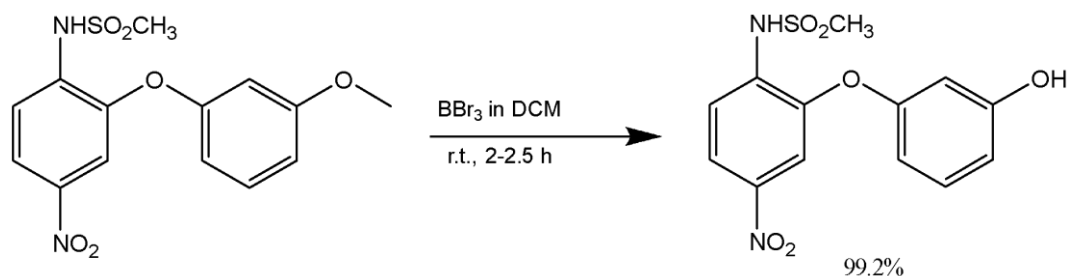
Scheme 1.27 – Synthesis of N -(2-(3-hydroxyphenoxy)-4-nitrophenyl)methanesulfonamide
